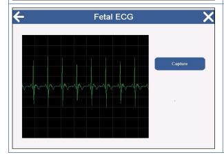
Example shown of an FECG screen trace displayed when it has found the fetal heart rate and established a connection.
